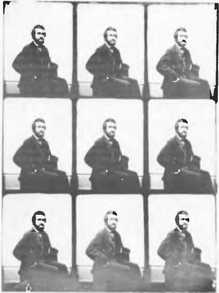
A single exposure with Wing's nine-lens shutter block produced an image like this on a 4-1/2 X 6 inch tintype plate. With proper masking and a series of steps and repeats however, the same lenses could easily make as many as 144 tiny images on the same plate.
